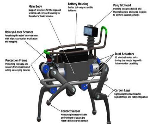
Fig. 2 Components of Autonomous Robot
