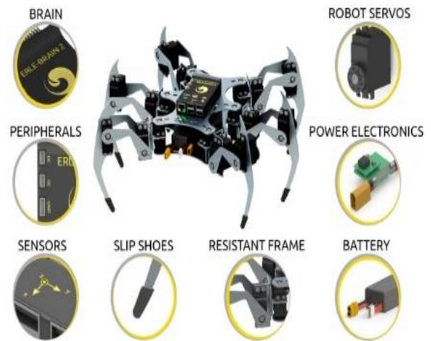
Fig. 1 Robots Components
