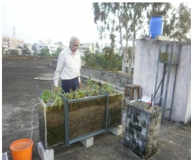
**Fig.2** The laboratory model of constructed Wetland along with constant flow rate arrangement system
