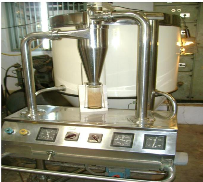
Figure 3: Co-current spray drier apparatus
